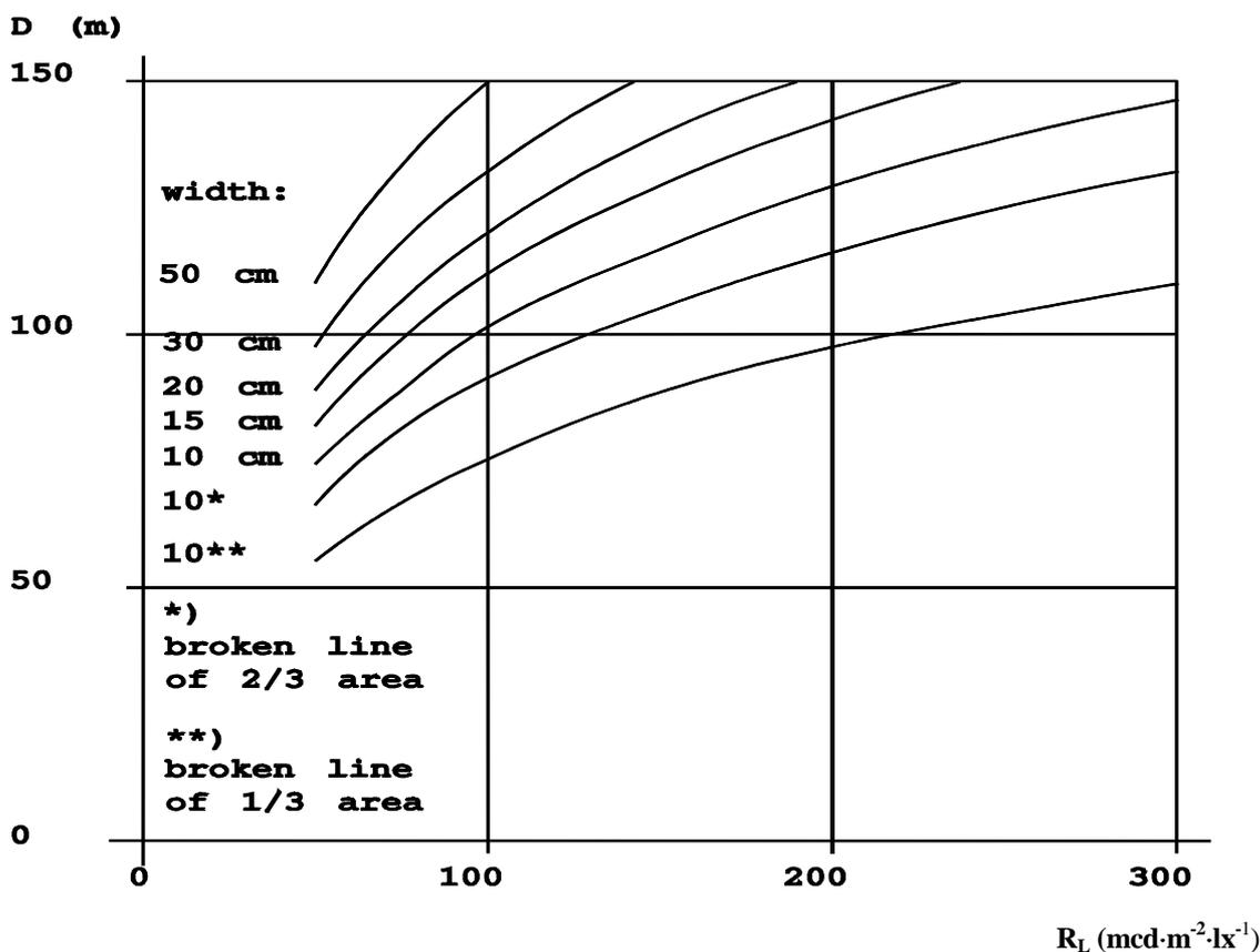
*Figure 5.1 - Visibility distance  $D$  for longitudinal road markings in high beam illumination.*
