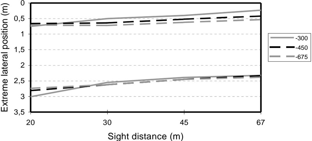
Figure 6.21 - Extreme lateral position of the wheels in left curve without clothoid at 90 km/h.
