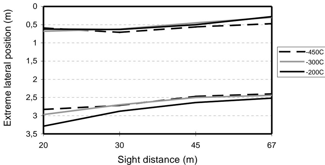
Figure 6.23 - Extreme lateral position of the wheels in left curve with clothoid at 90 km/h.
