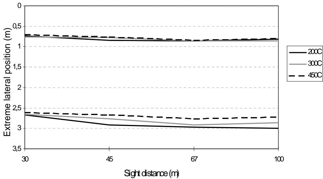
Figure 6.16 - Extreme lateral position of the wheels in right curve with clothoid at free choice of speed.
