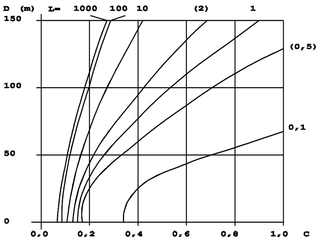
Figure 5.4 - Visibility distance ( $D$ ) for a continuous road marking of 10 cm width in uniform illumination.
