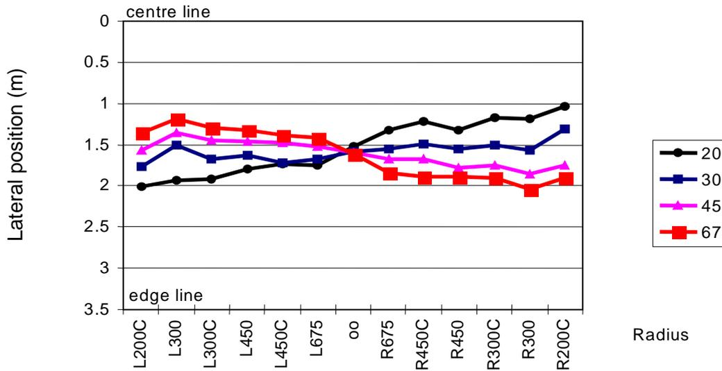
Figure 6.10 - Lateral position in every curve at the condition 90 [km/h] for different levels of sight distance.
