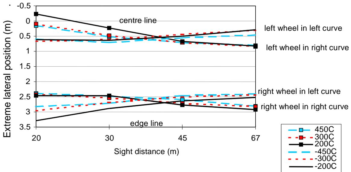
Figure 6.19 - Extreme lateral position of the wheels in curves with clothoid at the condition of cruise control.
