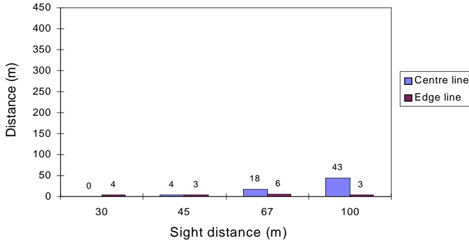
**Figure 6.25 - Distance driven on, or outside, road marking at own choice of speed.**
