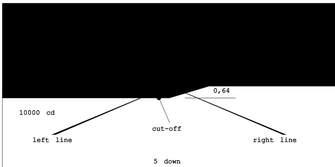
*Figure A4.4 - Intensity distribution of the low beam (shown for right-hand traffic).*
