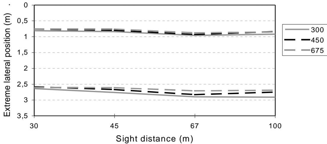
**Figure 6.14 - Extreme lateral position of the wheels in right curve without clothoid at free choice of speed.**
