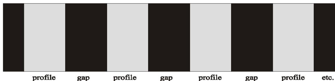
**B. Profiled road marking with gaps seen from the side**
