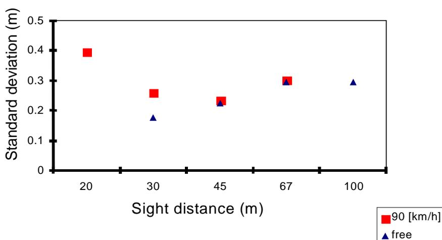
**Figure 6.24 - Standard deviation of lateral position at both speed conditions.**
