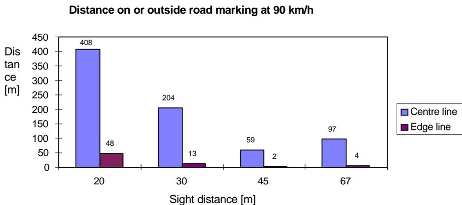
**Figure 6.26 - Distance driven on, or outside, road marking at 90 km/h**
