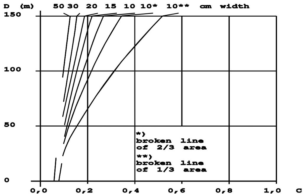
Figure 5.5 - Visibility distance ( $D$ ) for longitudinal road markings in full daylight ( $1.000 \text{ cd}\cdot\text{m}^{-2}$  of road surface).
