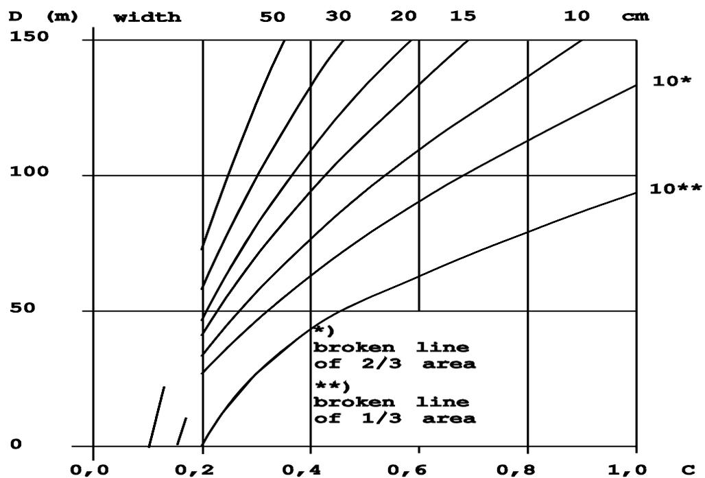
Figure 5.6 - Visibility distance ( $D$ ) for longitudinal road markings in typical road lighting for traffic routes ( $1 \text{ cd}\cdot\text{m}^{-2}$  of road surface).
