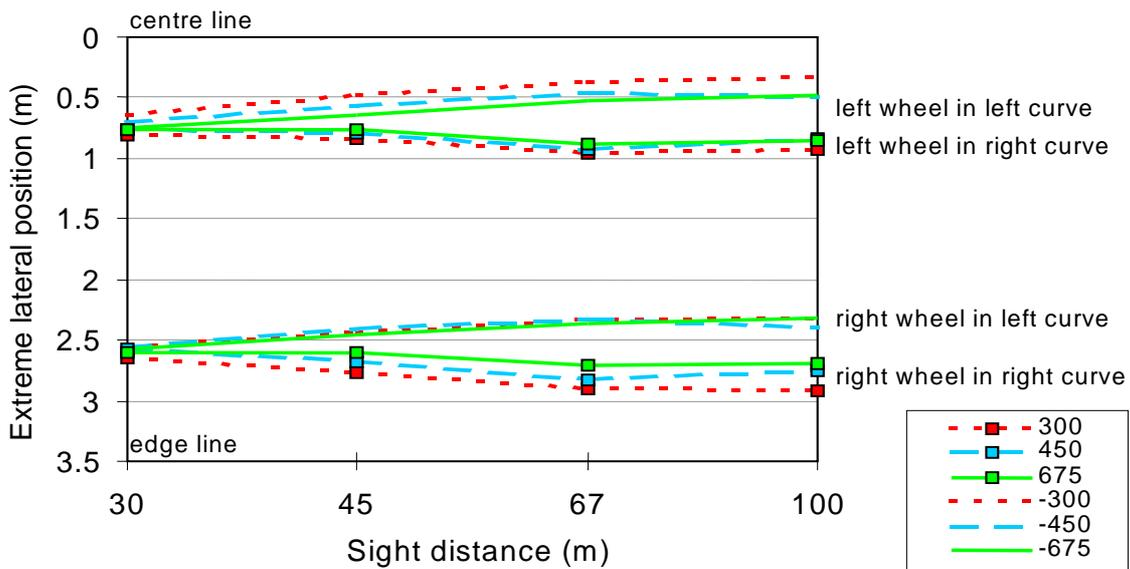
**Figure 6.12 - Extreme lateral position of the outside wheel in curves without clothoids at the condition of free choice of speed.**
