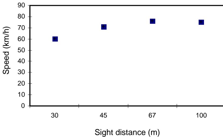
**Figure 6.3 - Mean speed (km/h), at free choice of speed, for the four levels of visibility of road markings.**
