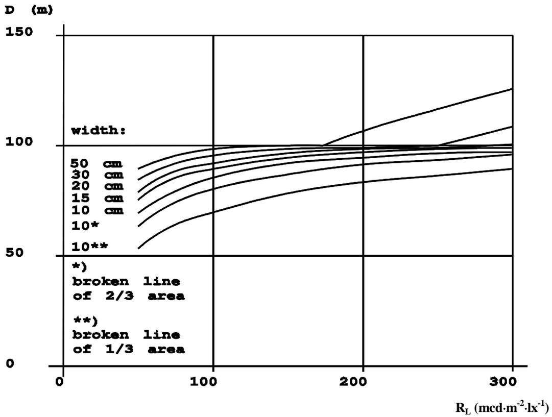
Figure 5.2 - Visibility distance ( $D$ ) for edge lines in low beam illumination.
