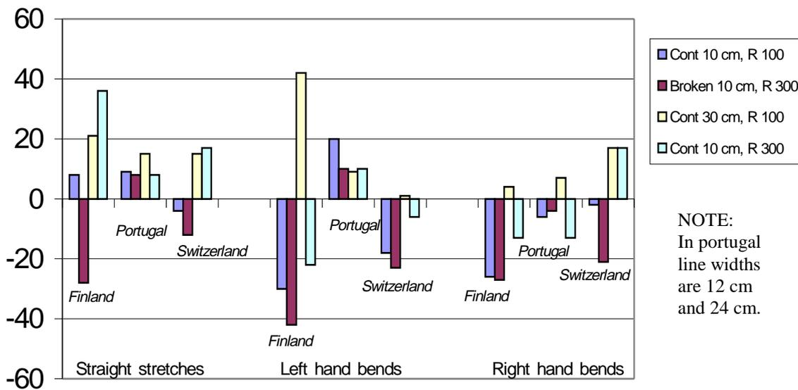
**Figure 7.5 - 99<sup>th</sup> percentile values of the change in the lateral position (cm) by road marking type.**
