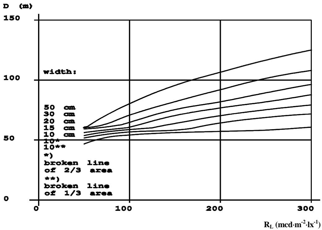
Figure 5.3 - Visibility distance ( $D$ ) for centre lines in low beam illumination.
