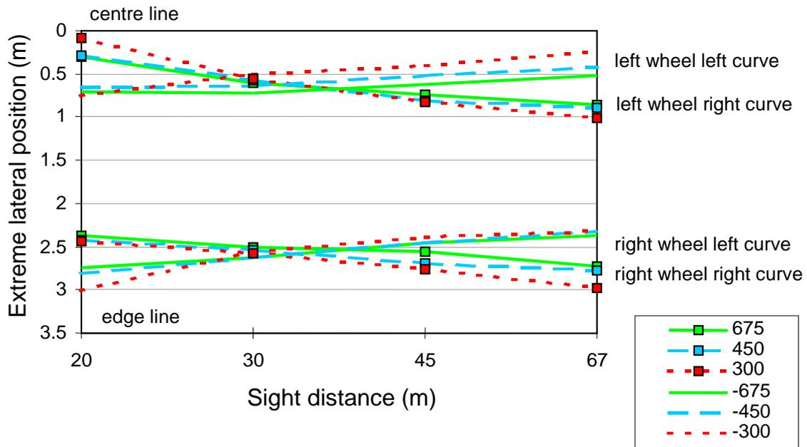
Figure 6.18 - Extreme lateral position of the outside wheel in curves without clothoids at the condition of cruise control.
