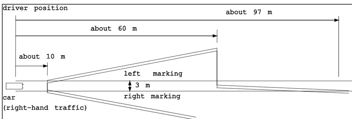
**Figure D.1 - Reach of the cut-off of low beam headlamps for a passenger car driving in a 3 m wide lane.**
