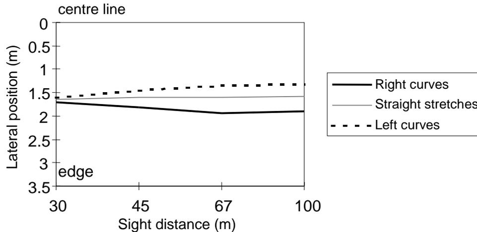
**Figure 6.6 - Mean lateral position for right and left curves and straight stretches at the condition free choice of speed.**
