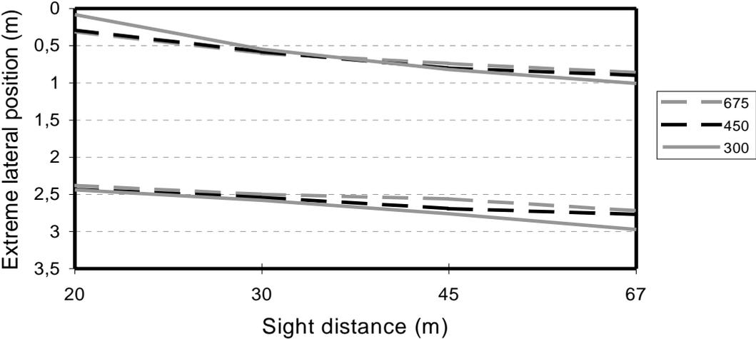
Figure 6.20 - Extreme lateral position of the wheels in right curve without clothoid at 90 km/h.
