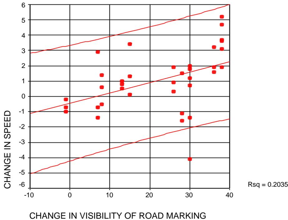
**Figure 7.7 - Relationship between the change in the visibility of road markings and the change in the mean travel speed level.**
