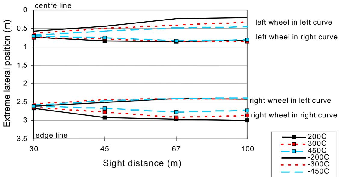
**Figure 6.13 - Extreme lateral position of the wheel in the curves with clothoids at the condition of free choice of speed.**
