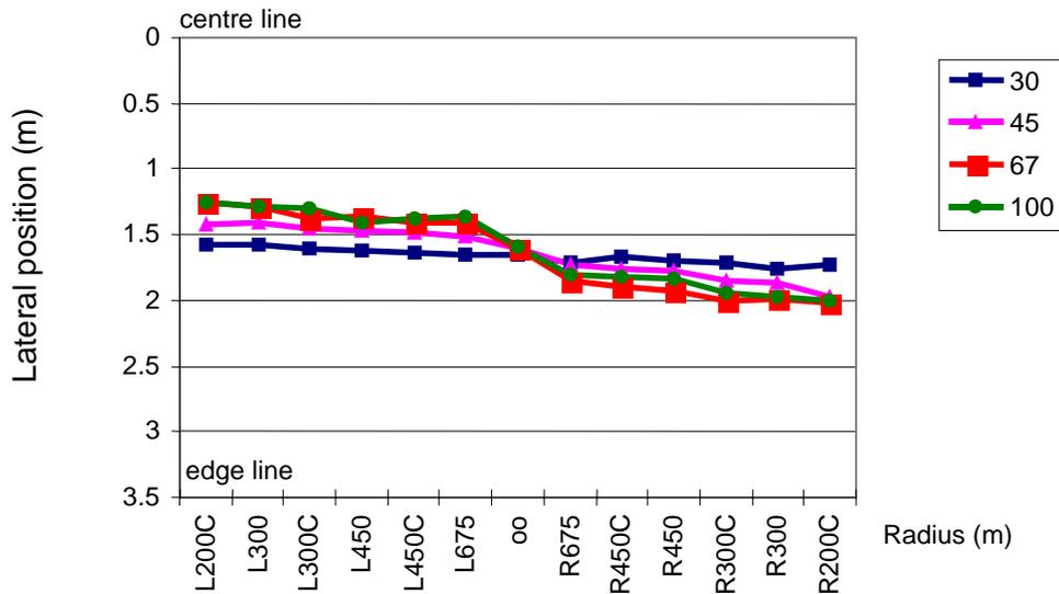
**Figure 6.7 - Lateral position in every curve at the condition of free choice of speed at the four levels of sight distance.**
