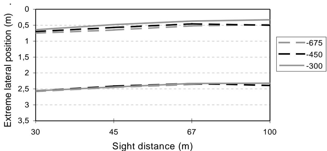
**Figure 6.15 - Extreme lateral position of the wheels in left curve without clothoid at free choice of speed.**
