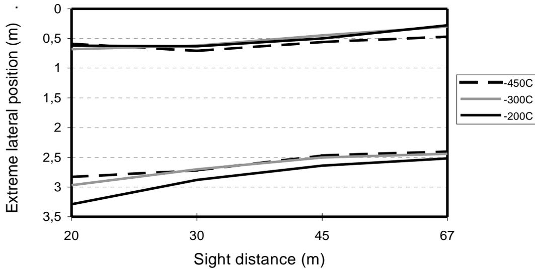
Figure 6.22 - Extreme lateral position of the wheels in right curve with clothoid at 90 km/h.
