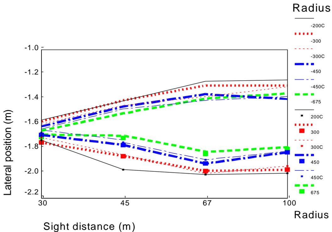
**Figure 6.8 - Lateral position for each type of curve at the condition of free choice of speed.**
